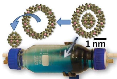
Fig. 19 A photograph of the flow systems with the blue “plume” from which the host-guest cluster crystallises (bottom). A schematic above is shown of the host-guest complex \{[\text{Mo}^{\text{VI}}_{36}\text{O}_{112}(\text{H}_2\text{O})_{16}]\subset[\text{Mo}^{\text{VI}}_{130}\text{Mo}^{\text{V}}_{20}\text{O}_{442}(\text{OH})_{10}(\text{H}_2\text{O})_{61}]\}^{22-} is shown in polyhedral plot (Mo centres shown in gold with the pentagonal centres shown in pink). Also, the ejection of the [\text{Mo}^{\text{VI}}_{36}\text{O}_{112}(\text{H}_2\text{O})_{16}]^{8-} template, to give the empty wheel, [\text{Mo}^{\text{VI}}_{130}\text{Mo}^{\text{V}}_{20}\text{O}_{442}(\text{OH})_{10}(\text{H}_2\text{O})_{66}]^{14-} , is shown (top).
