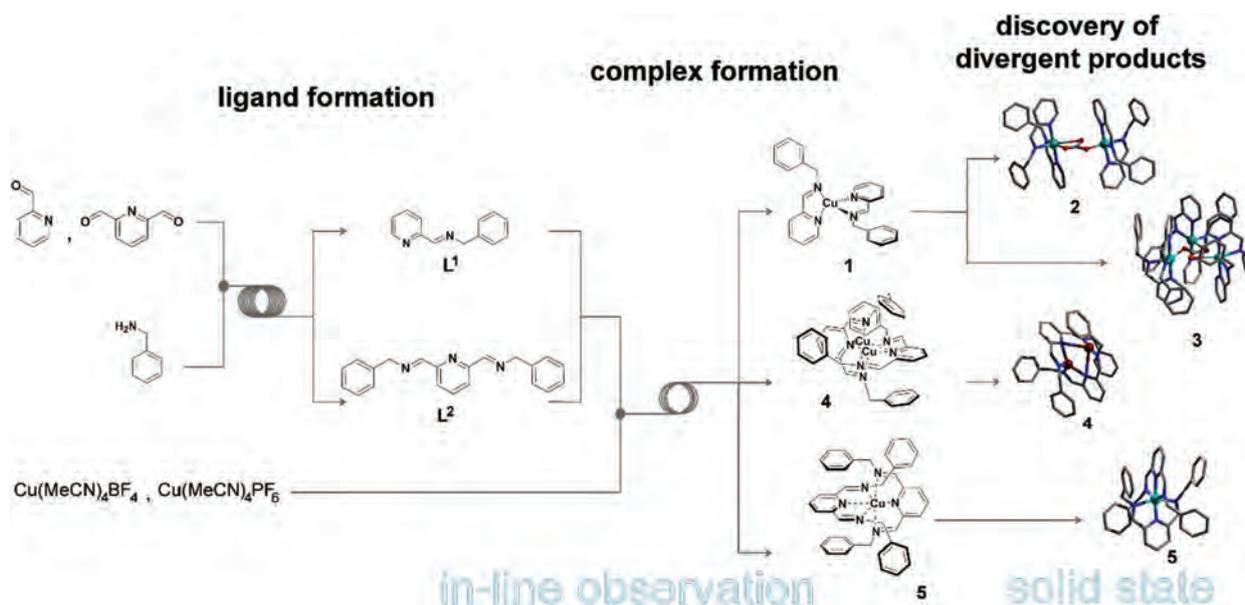
**Scheme 1** Flow synthesis of *N*-(2-pyridinylmethylene)-benzenemethanamine ( $\text{L}^1$ ), 2,6-bis(*N*-benzyliminomethyl)pyridine ( $\text{L}^2$ ) and their complexation with metal precursors  $\text{Cu}(\text{CH}_3\text{CN})_4\text{BF}_4$  and  $\text{Cu}(\text{CH}_3\text{CN})_4\text{PF}_6$ . See ESI† for full details.
