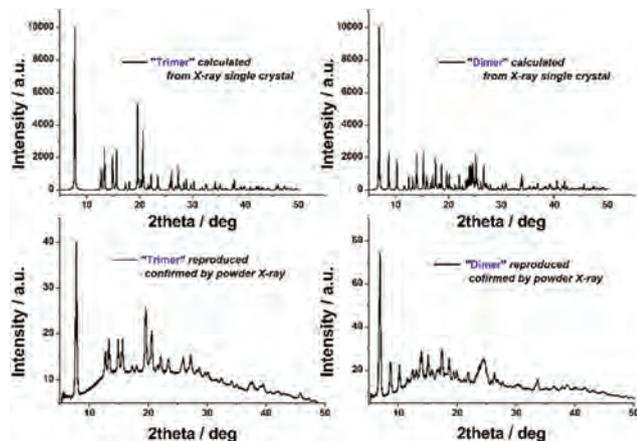
**Fig. 4** PXRD: top left: simulated pattern from single crystal  $[\text{Cu}_2(\text{L}^1)_4(\mu\text{-CO}_3)(\text{BF}_4)_2]$  (**2**), top right, simulated pattern from single crystal  $[\text{Cu}_3(\text{L}^1)_6(\mu\text{-CO}_3)(\text{PF}_6)_2(\text{OH})_2]$  (**3**), bottom left PXRD measurement of reproduced material **2**, bottom right, PXRD measurement of reproduced material **3**.
