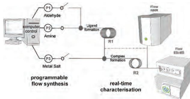
**Fig. 1** Schematic representation of the digital-programmable-flow-platform to perform ligand-complex synthesis in an automated way. The syringe pumps are computer controlled to deliver the chosen reagents in a well synchronized way into the flow reactors. New compounds are formed *in situ* and detected by real-time analyses.
