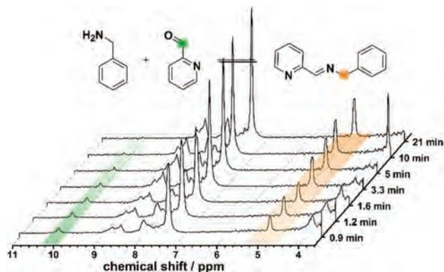
Fig. 2 Schematic of the real-time observation in the flow synthesis of  $L^1$  at different residence times showing a comparison of the normalised  $^1\text{H}$ -NMR spectra collected during the in-line benchtop NMR study.
