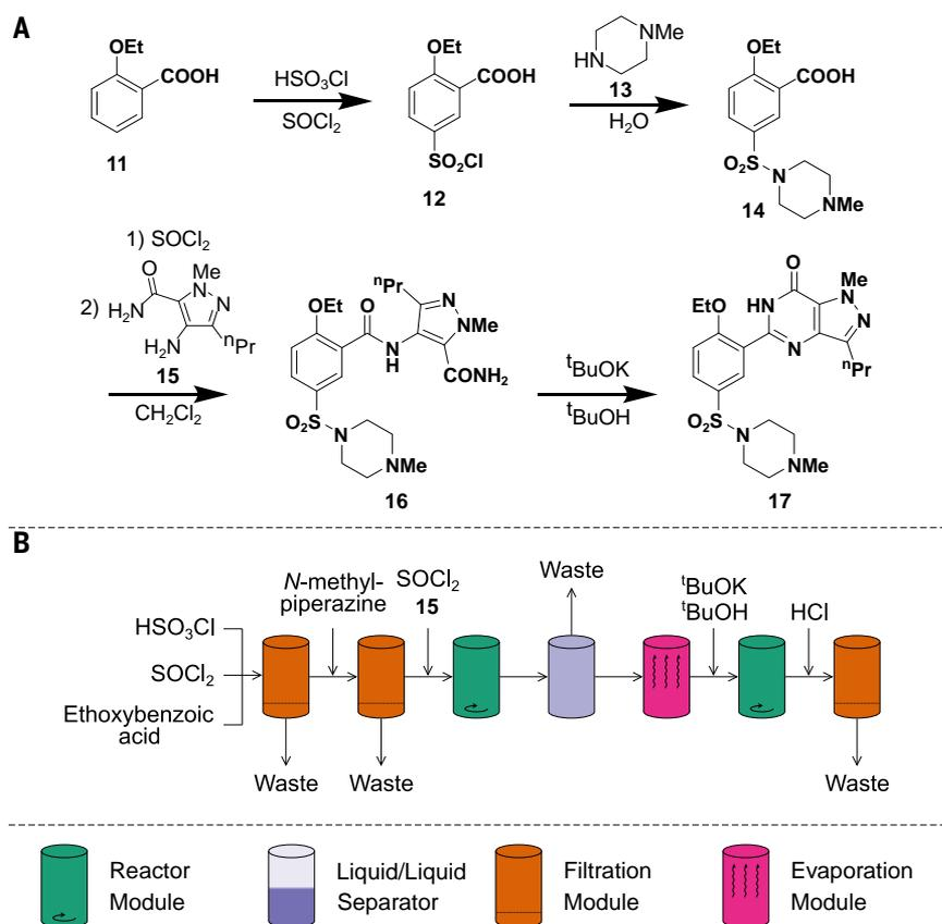
**Fig. 6. Synthesis of sildenafil (17).** (A) Synthetic route to sildenafil. <sup>t</sup>Bu, *tert*-butyl; <sup>n</sup>Pr, *normal*-propyl. (B) Sequence of unit operations required for the synthesis.
