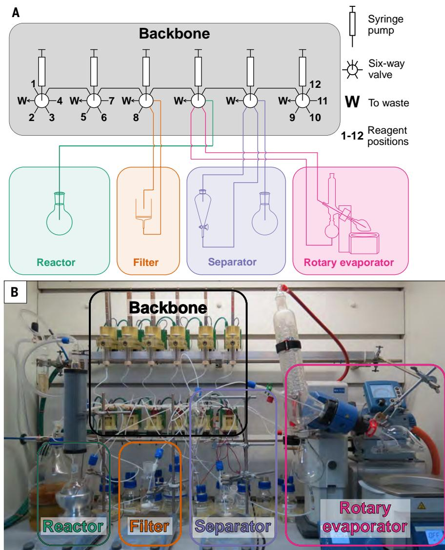
**Fig. 3. Physical implementation of the synthesis platform.** (A) Schematic representation of the Chemputer, highlighting modules used for four commonly encountered unit operations. The lines represent fluidic connections. (B) Photograph of one Chemputer setup used in this work. The various modules are highlighted in correspondence to the schematic.
