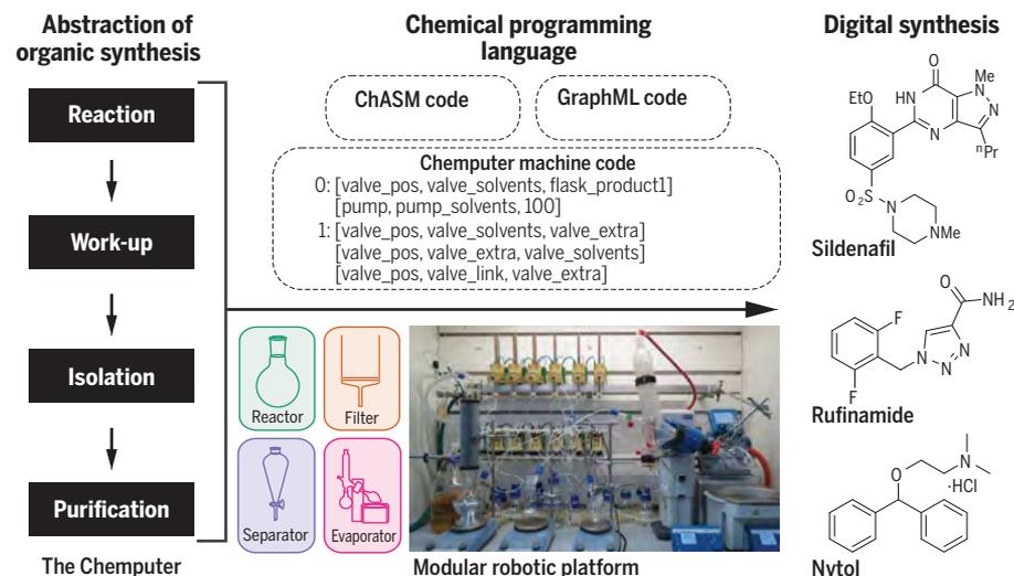
**Abstraction of organic synthesis to the Chemputer software and hardware standards.** The Chemputer system can perform multistep organic synthesis protocols on the bench by using a modular system with hardware and software standards.
