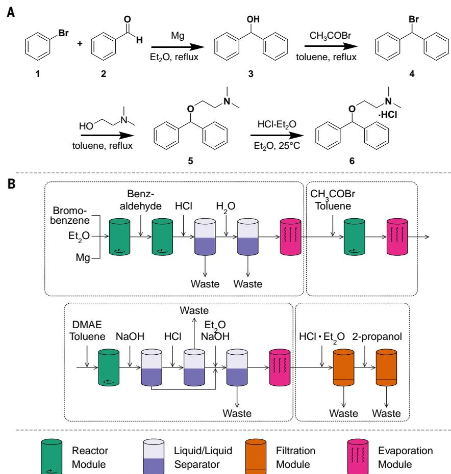
**Fig. 4.** Synthesis of diphenhydramine hydrochloride (**6**). (A) Modified synthetic route to diphenhydramine hydrochloride. Et, ethyl. (B) Sequence of unit operations required for the synthesis. The dotted boxes denote the four stages of the synthesis. DMAE, dimethylaminoethanol.
