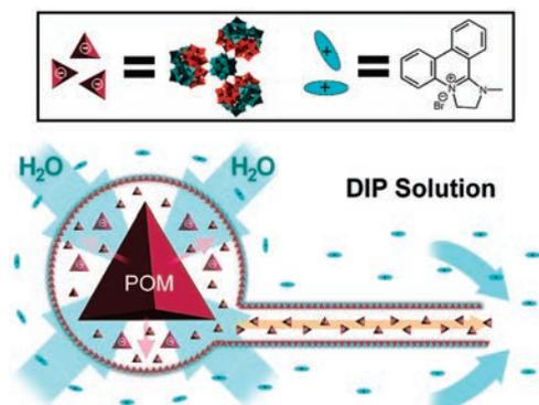
**Figure 1.** A schematic representation of the formation of micrometer-scale tubular structures from molecular building blocks, anionic POMs, and organic DIP cations. The arrows indicate the flow of DIP solution to the crystal and tube surface and the ingress of water into the membrane.
