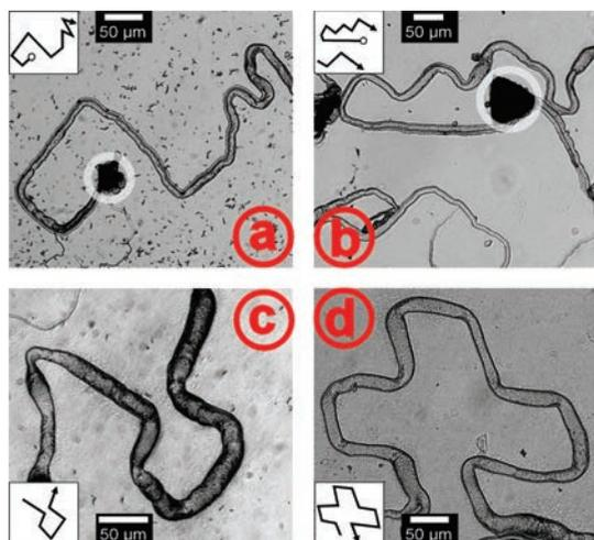
**Figure 2.** Motifs “drawn” by controlling the tube growth direction. (a) 90° bends followed by a series of 180° turns. (b) A series of 90° bends to make a zigzag motif. (c) 90° bends to form a square. (d) A series of 90° turns making a cross shape. Circles indicate the crystals from which tubes are growing. Inset diagrams show the direction of the tube growth.
