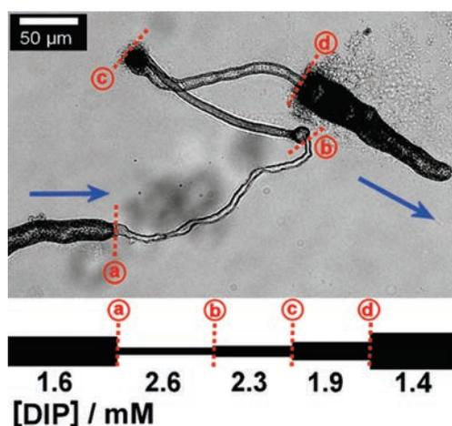
**Figure 3.** Size control of a growing tube by altering the available concentration of cations at points (a), (b), (c), and (d). The estimated concentrations at each point are shown in the lower section.
