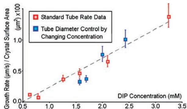
**Figure 4.** A plot of growth rate/crystal surface area against the overall concentration of DIP. Red squares show the linear trend increase in growth rate as the concentration is dropped, and blue squares show rate data for a tube where the concentration of DIP is varied while growing.
