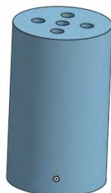
Supplementary Figure S8. 3d printed part to direct tubing output into vial.
