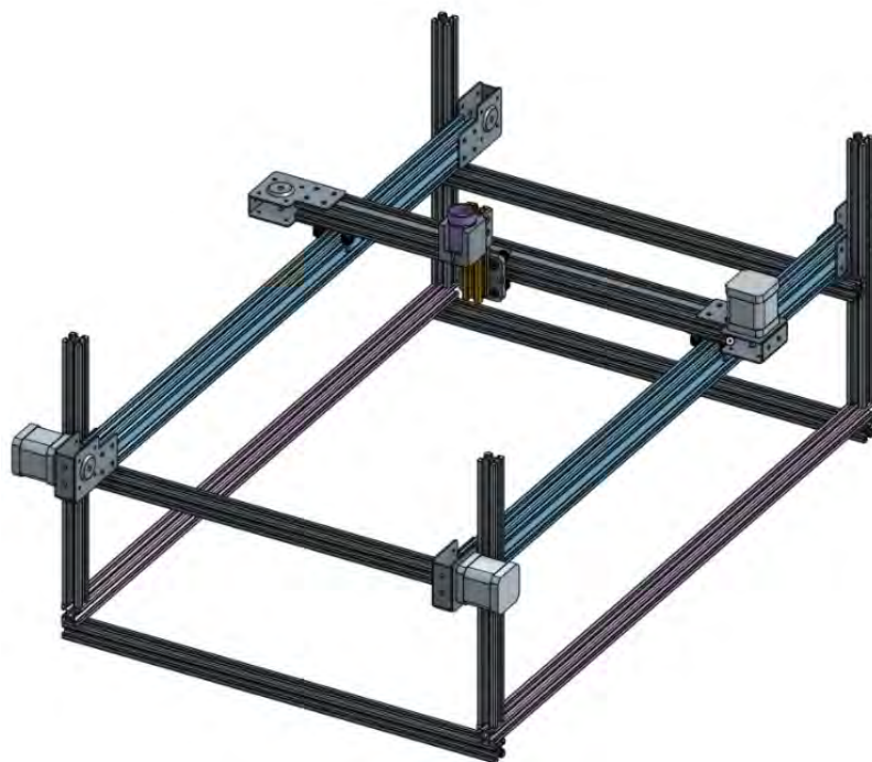
Supplementary Figure S5. Schematic of the lower half of the robot. The camera positioned on a mobile gantry (Supplementary Figure S6) is visible.
