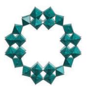
Fig. 3 Polyhedral structure of the tetrameric  $[Se_8W_{48}O_{176}]^{32-}$  wheel. (Colour code:  $\{Se_2W_{12}\}\$ units = teal polyhedra. Cations and water molecules have been omitted for clarity).
