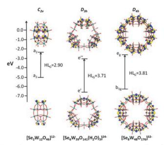
Fig. 4 Comparison of the frontier molecular orbitals of the {Se<sub>2</sub>W<sub>12</sub>} building block, 3 and 5 showing the positions and energies of the HOMO and LUMO states and the corresponding HOMO-LUMO gap (in eV).
