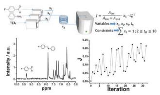
**Fig. 17** Self-optimisation platform employing in-line NMR. An acid catalysed imine synthesis was selected as a benchmark reaction to validate the platform. Ref. 43. Published by The Royal Society of Chemistry.
