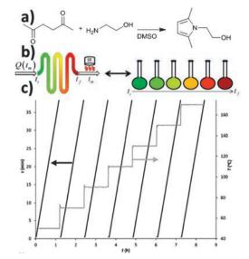
**Fig. 8** The treatment of a low dispersion microfluidic device as a series of batch reactors monitored by in-line ATR-IR allows for a quick determination of kinetic parameters. (a) Scheme of the Paal–Knorr employed as benchmark reaction. (b) Representative scheme of the time-series concept employing flow-rate gradients. (c) Example of a flow-rate, time and temperature series. Adapted from ref. 30. Copyright Wiley.
