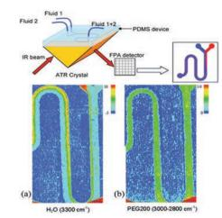
**Fig. 4** Up: Scheme of the microfluidic device coupled to an ATR-IR cell for IR imaging along the channels. Below: IR imaging of the mixture of (a)  $H_2O$  and (b) PEG200. Reproduced from ref. 25 with permission from The Royal Society of Chemistry.
