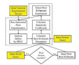
**Fig. 13** Flow diagram for the kinetic parameter estimation under continuousflow conditions. Reprinted with permission from ref. 44. Copyright 2012 American Chemical Society.
