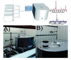
**Fig. 11** Low field benchtop NMR adapted as in-line analytics in a continuous-flow platform. Up: Schematic of the synthetic platform and examples of <sup>1</sup>H and <sup>13</sup>C acquired in flow. Down: Pictures of rig: general view (A) and details of the benchtop NMR (B). Reprinted from ref. 43. Published by The Royal Society of Chemistry.
