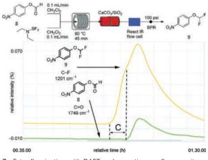
**Fig. 7** Ester fluorination with DAST under continuous-flow monitored by flow-IR. Up: Reactor and reaction scheme. Down: Relative intensity of the product 9 and unreacted ester 8 as a function of time. *C* represents the time delay between the detection of both compounds due to the chromatographic retention. Adapted with permission from ref. 26. Copyright 2010 American Chemical Society.
