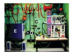
**Fig. 5** Continuous-flow reactor set-up with integrated ATR-IR analytics. A Vapourtec series reactor including HPLC pumps (A), a reactor coil (B), a packed bed column (C), the analytical flow cell (D) and the ReactIR spectrometer (E). Reprinted with permission from ref. 26. Copyright 2010 American Chemical Society.
