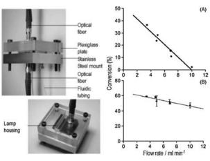
**Fig. 1** Left: Pictures of the microreactor designed and fabricated for photochemical transformations with integrated fiber optics for reaction monitoring by UV-Vis. Right: Conversion values observed for benzopinacole as a function of the flow rate by in-line UV-Vis (A) and HPLC (B). Reproduced from ref. 14 with permission from The Royal Society of Chemistry.
