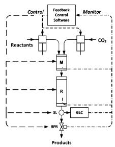
**Fig. 16** Schematic of a continuous-flow self-optimisation rig. The reactants and  $CO_2$  are pumped to a pre-heater and mixer (M) and into the reactor (R). A sample loop (SL) collects the product stream and sends it to the on-line gas-liquid chromatograph (GLC). The back-pressure regulator (BPR) maintains the system pressure. Reprinted with permission from ref. 13. Copyright 2011 American Chemical Society.
