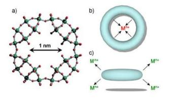
Figure 1. (a) Nanoporous  $[P_8W_{48}O_{184}]^{40-}$  structure, with simplified ring representation showing both (b) endocyclic (red) and (c) exocyclic (green) coordination of transition metals. Dark green spheres, W; red spheres, O; light blue rings,  $[P_8W_{48}O_{184}]^{40-}$ .
