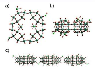
**Figure 4.** Ball-and-stick representation of the  $\{P_8W_{48}\}$  SBU in compound 3 from (a) top-down and (b) side-on. (c) "Planar chain" connectivity of POMzite-14(Ni) in one dimension. Dark green spheres, W; red spheres, O; light green spheres, Mn; dark blue spheres, P.
