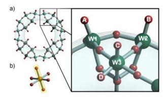
**Figure 5.** (a)  $\{P_8W_{48}\}$  ring-shaped SBU node, with close-up of the smallest repeating  $[P_{0.5}W_3O_{11.5}]^{2.5-}$  subunit, highlighting the three inequivalent W atoms and four inequivalent W=O<sub>T</sub> (labeled A, B, C, and D). (b) Octahedral  $\{TMO_6\}$  linker (TM = Mn, Co, Ni) which can be used to connect adjacent  $\{P_8W_{48}\}$  SBUs.
