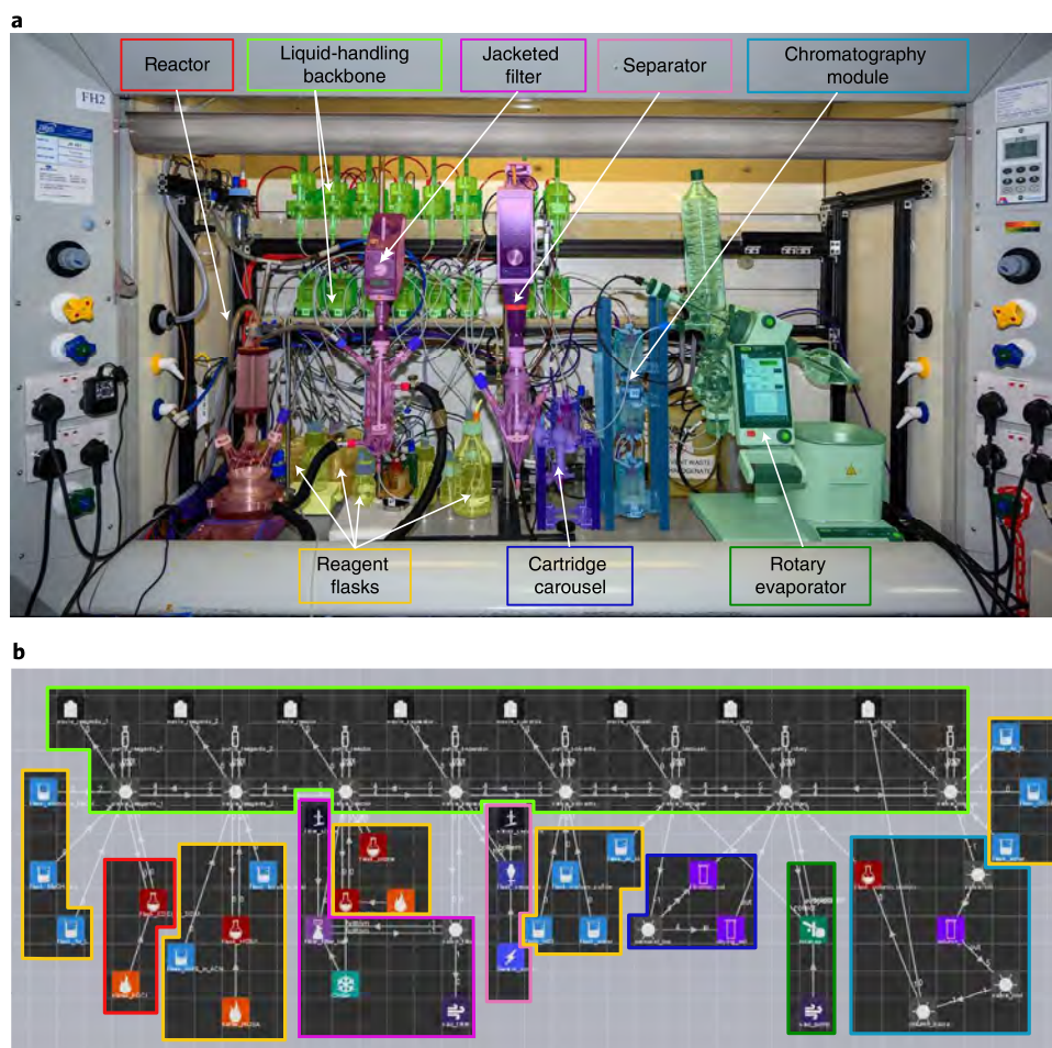
Fig. 5 | Implementation and topology of the synthesis platform. a , Physical instance of the Chemputer used for the synthesis of NHS-diazirine. The discrete modules are highlighted in different colours and labelled. b , Representation of the same instance in graph format; the modules are highlighted according to the colour code used in a .
