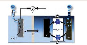
Fig. 2 Schematic of our polyoxometalate-based electrolyser system; reproduced from ref. 15.
