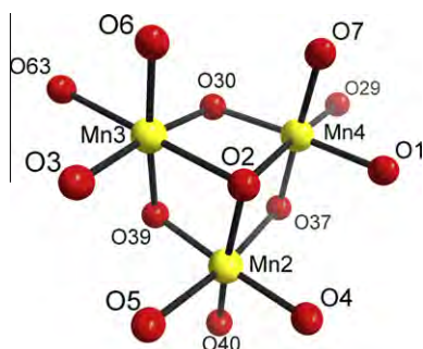
Fig. 3. Isolated core unit of [\text{Mn}^{\text{II}}_2[\text{Mn}^{\text{II}}(\text{H}_2\text{O})_5\text{Mn}^{\text{III}}_3(\text{H}_2\text{O})(\text{B}-\beta\text{-SiW}_9\text{O}_{34})(\text{B}-\beta\text{-SiW}_6\text{O}_{26})]_2]^{18-} 1a showing the truncated cubane core which is composed of three high-spin Jahn–Teller (JT) distorted Mn(III) centres bound by \mu_2\text{-O}^{2-} and \mu_3\text{-O}^{2-} anions. All Mn(III) ions are d^4 and six-coordinate: Mn2 is ligated to six oxo-ligands (three \mu_2\text{-O}^{2-} , two \mu_3\text{-O}^{2-} and one \mu_4\text{-O}^{2-} ), Mn3 is ligated to five oxo-ligands (two \mu_2\text{-O}^{2-} , two \mu_3\text{-O}^{2-} and one \mu_4\text{-O}^{2-} ) plus one \text{H}_2\text{O} ligand: \text{Mn}^{\text{II}}\text{O}_5(\text{OH}_2) ; while Mn4 is coordinated to six oxo-ligands (three \mu_2\text{-O}^{2-} and two \mu_3\text{-O}^{2-} and one \mu_4\text{-O}^{2-} ). All three Mn ions share O2, which is \mu_4\text{-O}^{2-} and bound also to Si. Colour scheme: manganese (yellow spheres) and oxygen (red spheres). (For interpretation of the references to colour in this figure legend, the reader is referred to the web version of this article.)
