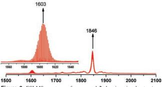
**Figure 3.** ESI-MS spectrum of compound **3** showing signals at m/z = 1847 and 1603.
