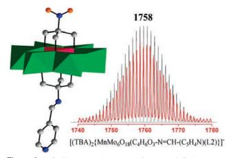
**Figure 2.** Left: X-ray crystal structure of compound **2** shown as a polyhedral representation showing that a pyridyl ring has been covalently tethered to the Mn-Anderson cluster (Mn, pink; Mo, green; N, blue; C, gray; O, orange). Right: ESI-MS spectrum of the molecular ion peak of compound **2** (actual spectrum in red; calculated spectrum in black).
