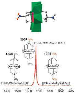
**Figure 1.** Top: One disorder part of the X-ray crystal structure of compound 1 in a polyhedral representation shows the nitro and amino groups capping both sides of the Mn-Anderson cluster (Mn, pink; Mo, green; C, gray; N, blue; O, orange; H, black). Below: ESI-MS spectrum of compound 1. The molecular ion peaks of the corresponding symmetric products at m/z = 1640 and 1700 that do not appear are shown.
