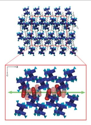
Fig. 3 Representation of the BTC-filled channels in 1. Top: View along the crystallographic b axis. Bottom: Cross-section through the channels. Emphasised in red, space-filling representation: stacked BTC molecules. The green arrow indicates the directionality of the channels. Sparteine and water molecules are omitted for clarity.
