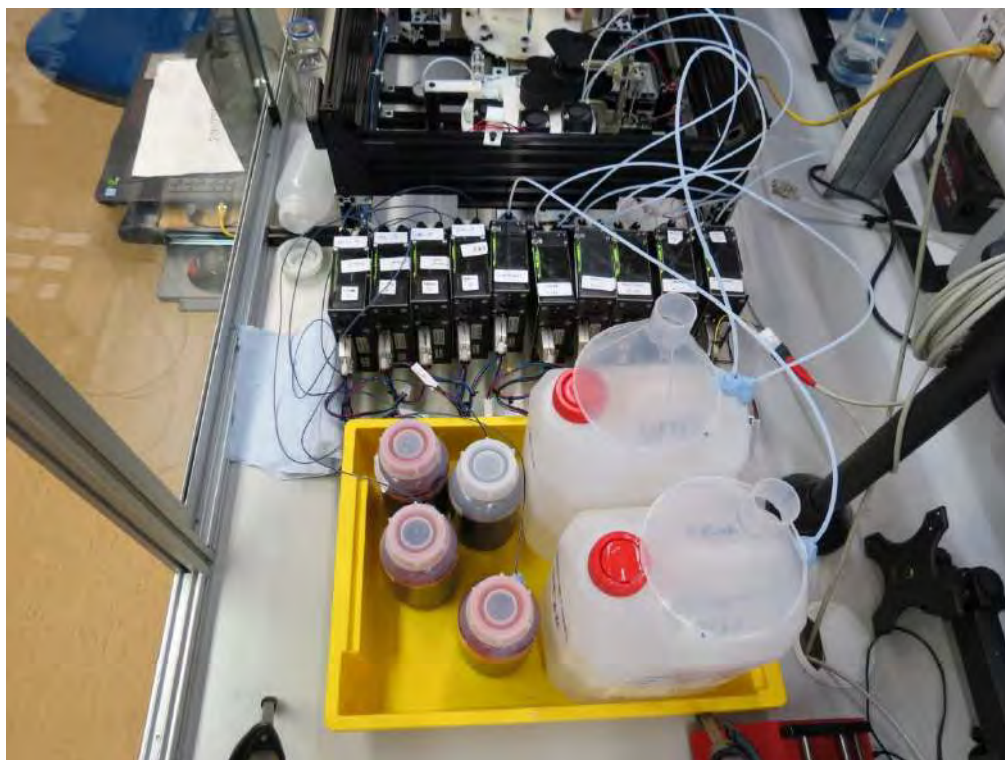
Supplementary Figure 55 – A photograph of the pumps and chemical inputs used for dropfactory.
