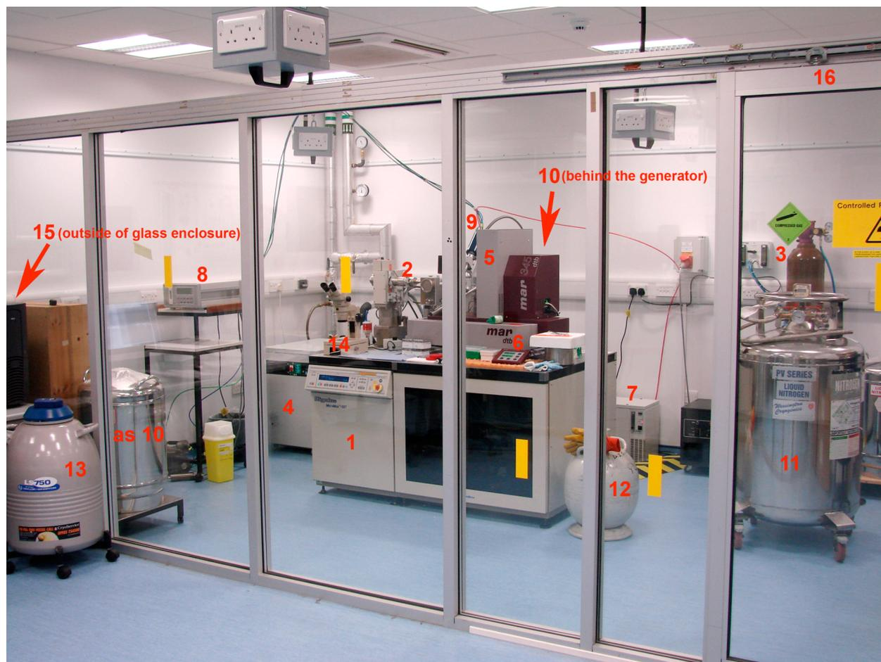
1. Rigaku X-ray generator MicroMax-007, micro-focus beam, 800-Watts (40kV/20mA) maximum power.
