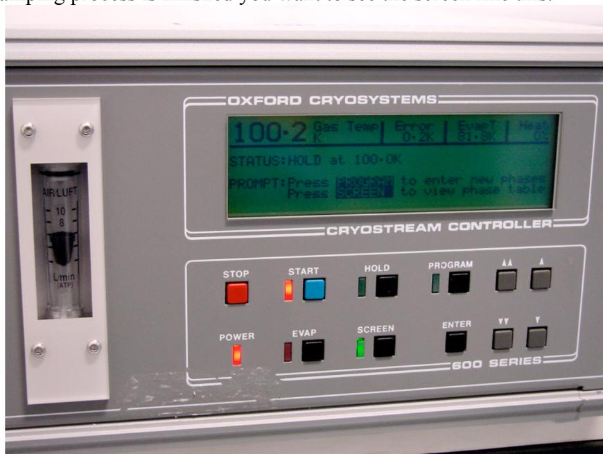
7. **Program the ramping-up process at the end of your work.** Choose one step ramping at the highest rate of 360 K/hr leading to a room temperature (290 K will do). When that is finished press button STOP, then switch off the POWER button at the back of controller. Finally, **switch the Dry Air unit off as well.**
