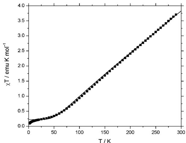
**Figure 3.** Temperature dependency of  $\chi T$  for **1** at 0.1 Tesla. Experimental values are represented by squares; the fit to an  $\text{Fe}^{\text{III}}_2$  Heisenberg model is shown by a gray line.
