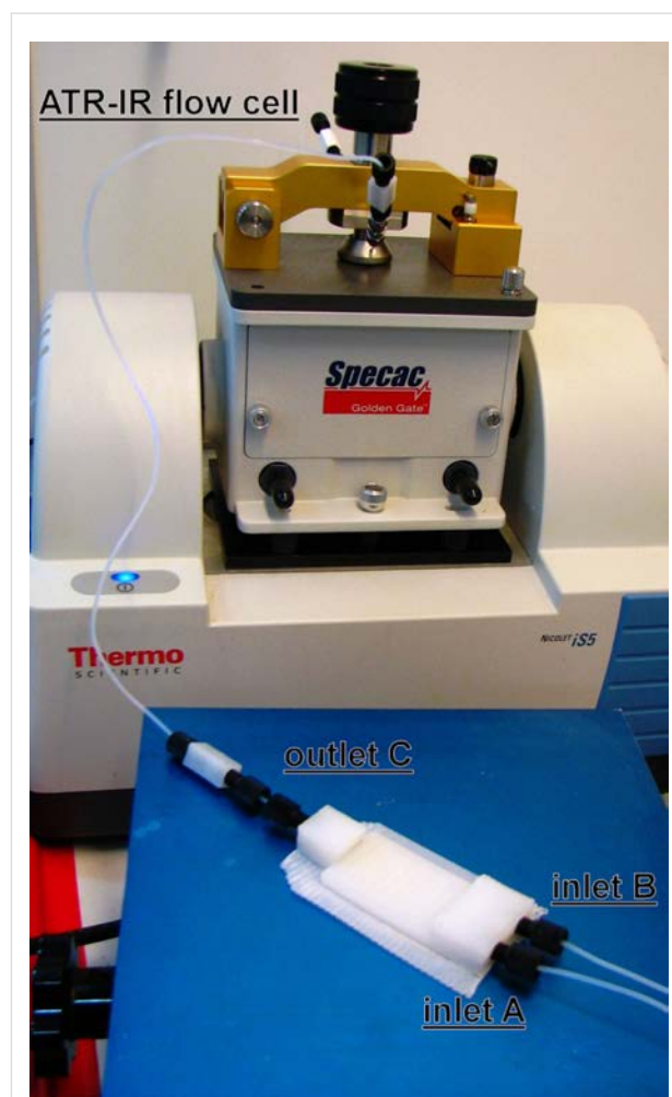
Figure 2: Flow system setup, where a R1 is connected to the syringe pumps and the ATR-IR flow cell with standard connectors.
