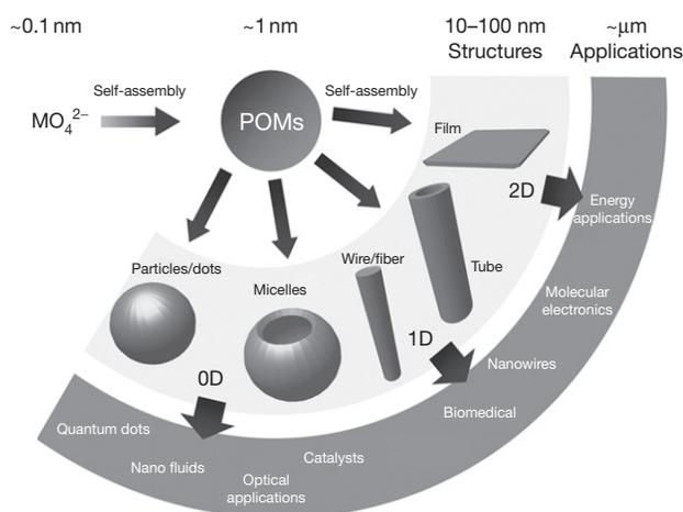
**Figure 31** POM clusters ( $\sim 1\text{--}5$  nm in size) are assembled from mononuclear metal-oxide ions ( $\sim 0.1$  nm of size) and can also act as building blocks for nanoscale structures through template-mediated and electrostatic self-assemblies.
