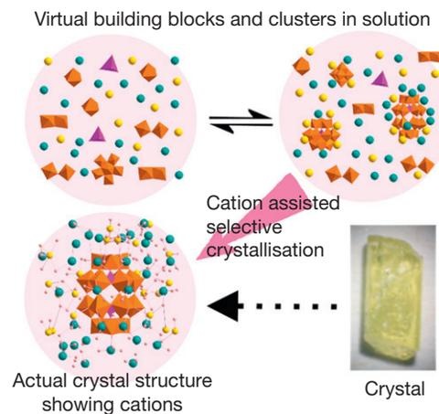
**Figure 7** The formation of various structural archetypes in solution highlighting the role of cations in selective crystallization of a particular product. Yellow and green spheres represent different cations. The top left shows a range of 'virtual' geometrically possible units and the top right shows the cations complexing the clusters and pulling certain structures out of solution. The orange polyhedra represent the metal addenda, in this case W.
