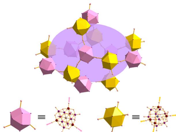
**Figure 25** Illustration of the nanosized pockets in  $[(\text{C}_4\text{H}_{10}\text{NO})_{40}(\text{W}_{72}\text{Mn}_{12}\text{O}_{268}\text{Si}_7)_n]$  highlighted by the purple ellipsoid (dimensions:  $\sim 2.7 \times 2.4 \times 1.3$  nm). The trigonal (rose) and tetrahedral (yellow) building block connectors are shown at the bottom; rose and yellow arrows highlight the connecting modes.
