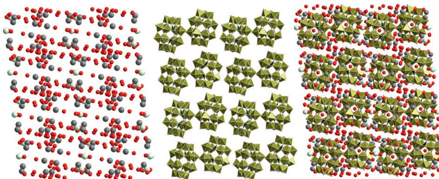
**Figure 8** Packing diagrams depicting the separate and combined arrangements of cations and anionic POM clusters in a crystal lattice. Left: Only cations (pale green and gray spheres) and solvent water molecules (red spheres); middle: only POM clusters (yellow and green polyhedra) and; right: POM cluster anions, counter-cations and solvent water molecules together in a crystal lattice.
