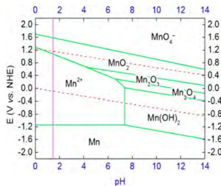
**Figure 6.** Simplified Pourbaix diagram for manganese in aqueous solution. Green lines represent the borders of thermodynamic stability of the various species (adapted from ref 24). Dissolved species are considered as having an activity of 1. Red dashed lines mark the region of water stability, the lower line corresponding to the hydrogen evolution reaction and the upper line to the oxygen evolution reaction. The vertical magenta line is drawn at pH = 1.6 as a guide to the eye.
