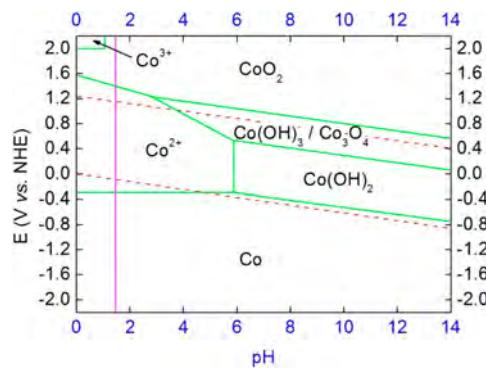
**Figure 1.** Simplified Pourbaix diagram for cobalt in aqueous solution. Green lines represent the borders of thermodynamic stability of the various species (adapted from ref 24). Dissolved species are considered as having an activity of 1. Red dashed lines mark the region of water stability, the lower line corresponding to the hydrogen evolution reaction and the upper line to the oxygen evolution reaction. The vertical magenta line is drawn at pH = 1.6 as a guide to the eye.
