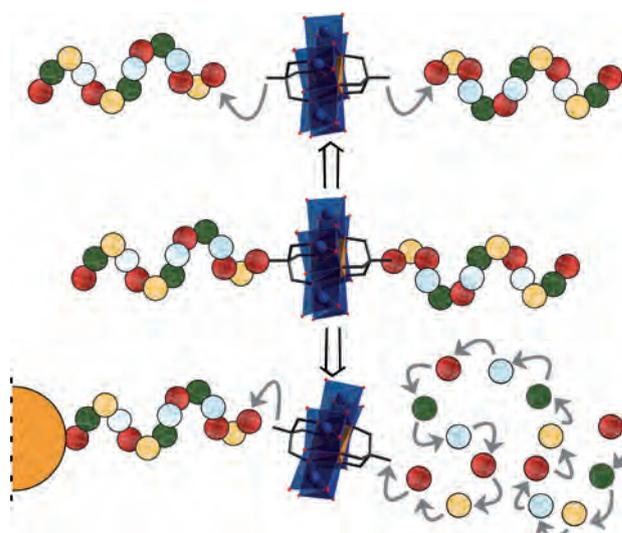
**Scheme 1.** Schematic representation of the two approaches that were considered for the integration of POM clusters into peptide chains: solution-phase reaction with pre-synthesized peptides (top) and incorporation of the POM building block as an unnatural amino acid during stepwise peptide synthesis (bottom).
