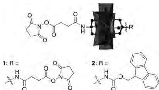
**Figure 1.** Mn-Anderson precursors **1–2** activated as NHS esters. Polyhedral/ball and stick representation of the Mn-Anderson  $[\text{MnMo}_6\text{O}_{18}(\text{O}(\text{CH}_2)_3\text{C})_2]^{3-}$  core;  $\text{MnO}_6$  and  $\text{MoO}_6$  are shown as light grey and black octahedra, respectively, and carbon atoms are depicted as black spheres; counteranions were omitted for clarity.
