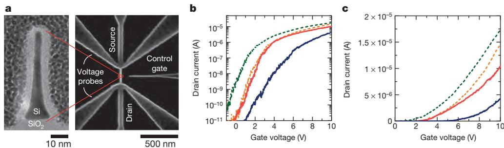
**Figure 2 | Image of the flash memory device and the drain current behaviour with an applied voltage to the control gate.**
