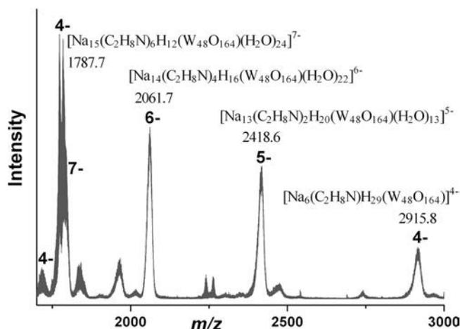
**Figure 5.** Negative mode mass spectrum of **1** in the *m/z* range of 1700–3000 showing the major envelopes labeled 4– to 7– corresponding to sequentially charged quasi-molecules of {W<sub>48</sub>O<sub>164</sub>}. The 7– overlaps with other lower mass signals of charge 4–. Representative assignments are provided in the Figure and Table S5 (SI).
