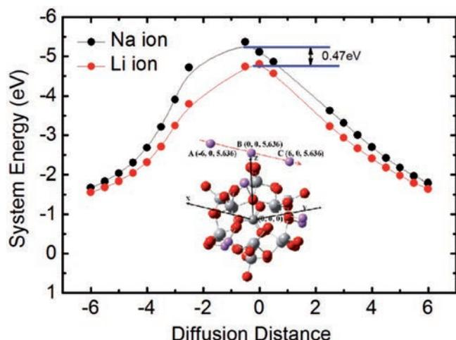
**Figure 3.** DFT calculations of the transfer energy barrier of  $\text{Li}^+$  and  $\text{Na}^+$  during the migration versus cation diffusion distance in  $\{\text{V}_{15}\text{O}_{36}(\text{CO}_3)\}$ . The inset picture shows the migration model for  $\text{Li}^+$  and  $\text{Na}^+$  cations in  $\{\text{V}_{15}\text{O}_{36}(\text{CO}_3)\}$ . The coordinate of the carbon atom in  $\text{CO}_3^{2-}$  was defined as a coordinate origin (0, 0, 0).
