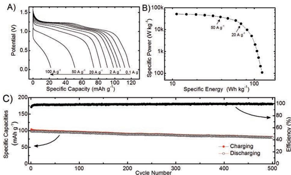
**Figure 2.** The electrochemical performance of a symmetric  $\text{Li}_7[\text{V}_{15}\text{O}_{36}(\text{CO}_3)]$  device A) discharge curves at 0.1, 0.2, 0.5, 1, 2, 5, 10, 20, 50, and 100  $\text{A g}^{-1}$ , respectively, B) specific power versus specific energy, C) long cycling performance at 1  $\text{A g}^{-1}$ .
