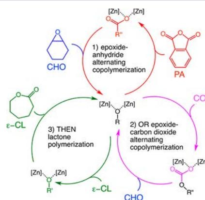
**Figure 8.** Example of chemoselective emergence of a sequence-controlled copolymer from a mixture of competing monomers determined by the electron-withdrawing strengths of substituents in ring-opening polymerization. Adapted from ref 38. Copyright 2016 American Chemical Society.
