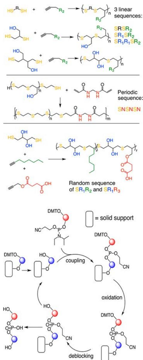
**Figure 3.** Click approaches used in producing sequence-controlled polymers. (top) Thiol–yne coupling in step-growth polymerization. Adapted from ref 11. Copyright 2014 Macmillan Publishers Ltd. (bottom) Phosphoramidite chemistry in a multistep-growth process. Adapted from ref 22. Copyright 2016 American Chemical Society.
