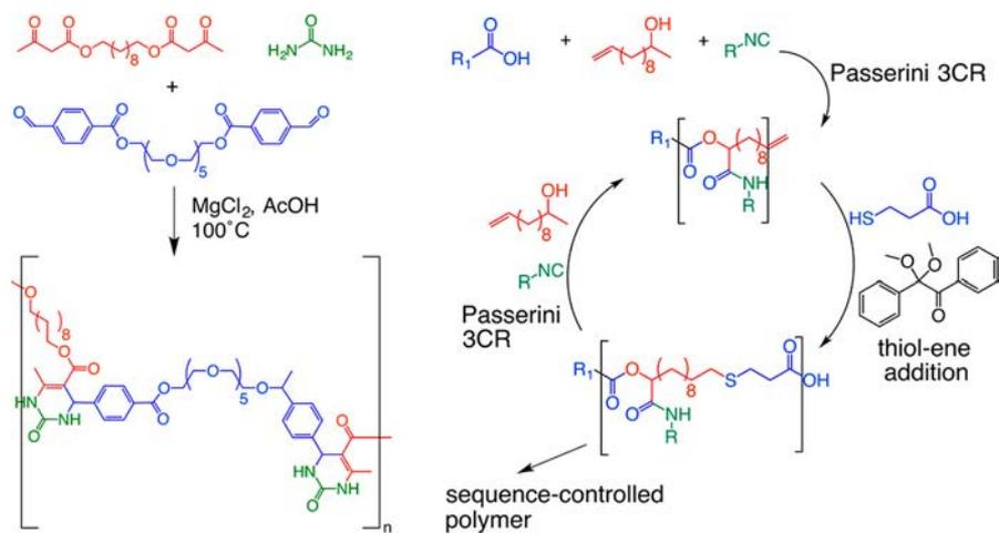
**Figure 4.** Three-component (left) Biginelli (adapted from ref 12; copyright 2016 American Chemical Society) and (right) Passerini (adapted with permission from ref 13; copyright 2014 Wiley) reactions and their utility for controlling sequence in step-growth polymerization.
