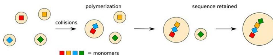
**Figure 6.** Collisions of monomer-containing droplets in a specific sequence leading to retention of that sequence in the resulting polymer.
