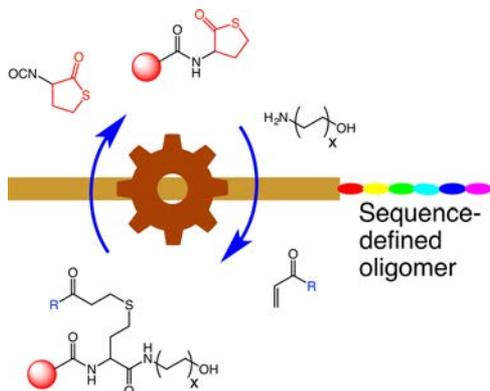
**Figure 11.** Operational principle of an automated system inspired by peptide synthesizers and used to produce sequence-defined oligomers. Adapted from ref 50. Copyright 2016 American Chemical Society.
