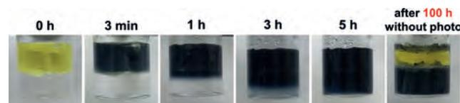
**Figure 3.** Color changes of the solution during Xe light irradiation from 0–5 h, membrane stability demonstrated by leaving the membrane for 100 h without irradiation. Upper phase;  $\text{MV}$ ,  $[\text{Ru}(\text{bpy})_3]\text{Cl}_2$ , TEOA (solvent; Bis-Tris buffer), Lower phase;  $\text{H}_3[\text{PW}_{12}\text{O}_{40}]$  (solvent; MilliQ).
