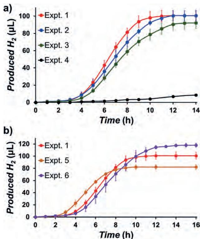
**Figure 4.** Time-courses of volume of hydrogen produced during photo-reaction a) at various Pt concentrations [Expt. 1 = 4.3, Expt. 2 = 2.6, Expt. 3 = 0.9 & Expt. 4 = 0  $\mu\text{M}$  wrt total solution volume], and b) at various  $\text{H}_3[\text{PW}_{12}\text{O}_{40}]$  concentrations [Expt. 5 = 5.3, Expt. 1 = 6.7 & Expt. 6 = 8.0 mM wrt total solution volume].
