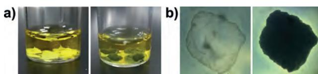
**Figure 2.** a) Photographs of iCHELLs composed of 100 mM  $[\text{PW}_{12}\text{O}_{40}]^{3-}$  in 25 mM  $\text{MV}^{2+}$  before (left), and after (right) 1 h light irradiation. b) Micrographs of one iCHELL (conditions as above) before (left) and after (right) 1 h light irradiation. The iCHELLs shown are approximately 3 mm in diameter.
