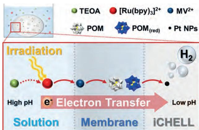
**Figure 1.** A schematic representation of photo-driven HER with iCHELLs and multi-step electron transfer across the membrane. The four component HER system comprises a photosensitizer ( $[\text{Ru}(\text{bpy})_3]^{2+}$ ), electron mediator (methyl viologen ( $\text{MV}^{2+}$ )), a catalyst (Pt colloid), and a sacrificial electron donor (triethanolamine (TEOA)). The iCHELL is constructed from POM anions, which also facilitate electron transfer across the membrane.
