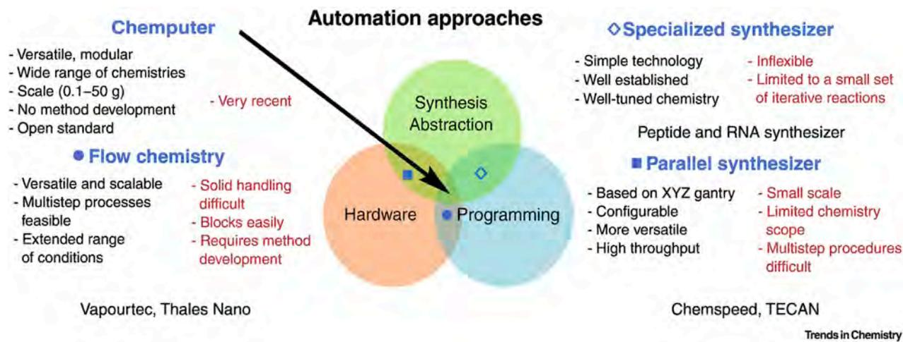
**Figure 1. Approaches to Automate Organic Synthesis: Specialized Synthesizer, Parallel Synthesizer, Flow Chemistry, and ‘the Chemputer’.**
