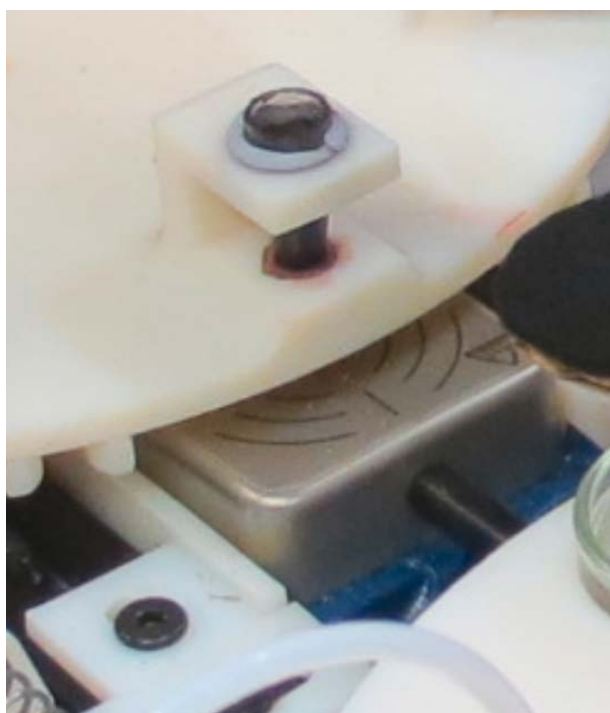
Supplementary Figure 58 - A photograph of the oil stirring station, with the small magnetic stirrer plate (silver) visible below the Geneva wheel.
