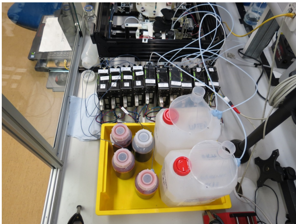
Supplementary Figure 54 – A photograph of the pumps and chemical inputs used for dropfactory.
