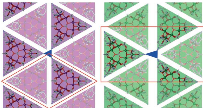
**Figure 2.** Comparison of the packing of  $\{\text{M}_{12}\}$  clusters in **1** (left, hexagonal system) and **2** (right, orthorhombic system) within the crystallographic  $ab$  plane. Red lines show the unit-cell boundaries and blue triangles are used to highlight the geometrical relationship enforced by hydrogen bonding between adjacent clusters. Colors are as in Figure 1.
