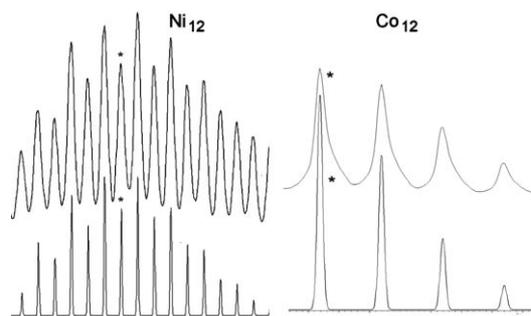
**Figure 5.** Cryospray mass spectrum for the  $\{\text{M}_{12}\}$  clusters at  $-40^\circ\text{C}$ . Experimental (top) and simulated data (below). Right:  $[\text{Co}_{12}(\text{OH})_{12}(\text{CH}_3\text{CO}_2)_{10}(\text{CO}_3)(\text{H}_2\text{O})_6(\text{tach})_6(\text{H})_1]^+$ ; \* = 2445. Left:  $[\text{Ni}_{12}(\text{CH}_3\text{O})_{12}(\text{CH}_3\text{CO}_2)_9(\text{CO}_3)(\text{tach})_6]^+$ ; \* = 2442 (simulated and experimental within 1 Dalton).
