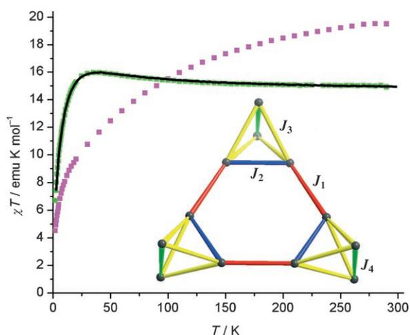
**Figure 3.** Temperature dependence of  $\chi T$  for **1** (purple squares) and **2** (green squares) at 0.1 T with the best fit to a Heisenberg model for **2** (black line). Inset: Assignment of the exchange parameters  $J_{1-4}$  to the  $M_{12}$  spin array:  $J_1$  red,  $J_2$  blue,  $J_3$  yellow,  $J_4$  green, see text for details.
