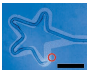
Figure 5. Automated control of the laser spot is possible, by using image analysis to track the end of the tube and keep the laser spot a constant distance ahead of the growth (circle). This enables us to assemble structures along predefined tracks (pale overlay). Scale bar: 500 \mu\text{m} .
