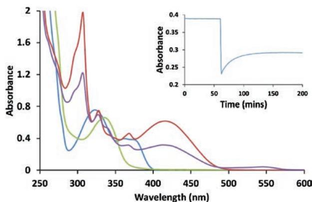
**Fig. 1** Spectra for the products, reactants and reaction mixture for the reaction between 0.1 mM BEP solution (2 mL, 1 eq) and 0.1 mM 3-aminofluoranthene and triethylamine solution (2 mL, 1 and 3 eq. respectively) (i) 0.1 mM BEP, blue curve; (ii) 0.1 mM 3-aminofluoranthene, red curve; (iii) product solution after 10 h, purple curve; (iv) 0.05 mM pseudo base, green curve. (Inset) Plot of absorbance changes at 373 nm against time.
