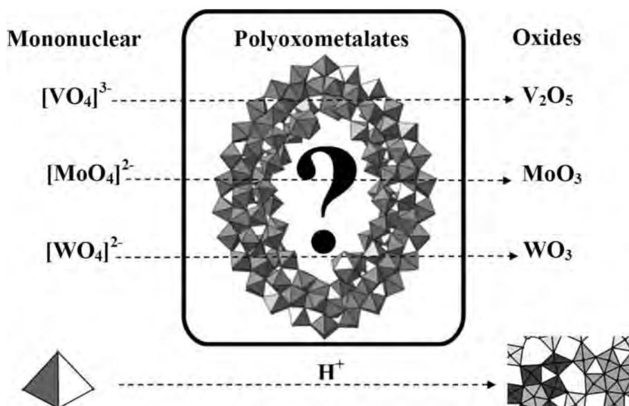
**Fig. 8** Polyoxometalates are formed in experimental conditions that allow linking of polyhedra. Discrete structures are formed as long as the system is not driven all the way to the oxide. One such example, in this case a part of an  $\{\text{Mo}_{256}\text{Eu}_8\}$  cluster unit, is depicted in the square.
