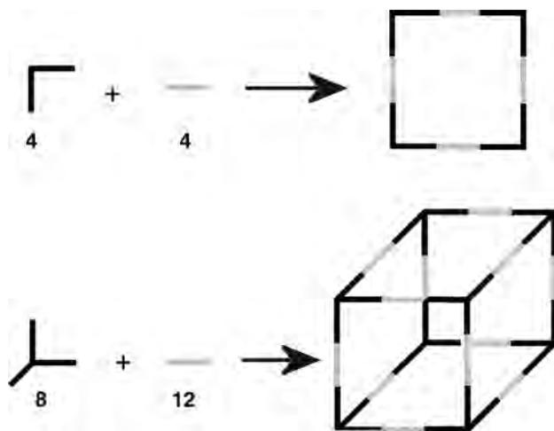
**Fig. 2** A schematic showing the assembly of a square and a cube, which require 2D and 3D 90° corner units, respectively, linked by linear spacers.
