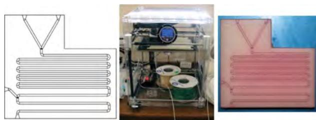
**Fig. 1** (Left) Schematic drawing of the design of one of the reactors used in this study. (Centre) 3DTouch™ 3D printer used in the fabrication of the micro- and milli-reactors. (Right) device printed from the drawing shown on the left. The channels in the device have been filled with a methanol solution of Rhodamine B dye to render them visible, and the dye can be completely removed by subsequent washing.
