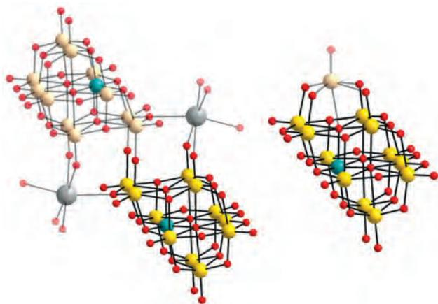
**Fig. 4** Ball and stick models showing a comparison between the structure of the  $K^+$  stabilised  $[K_2(MnV_{11}O_{32})]^{8-}$  dimer<sup>14,15</sup> (left) and compound **1** (right). The undecavanadate building unit common to both compounds has been highlighted in each case. Colour code: V = yellow/tan, Mn = teal, K = grey, O = red.
