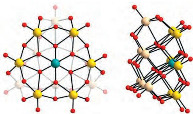
**Fig. 1** Ball and stick representation of the  $[\text{MnV}_{12}\text{O}_{34}]^{4-}$  cluster in **1**. Left: top down view highlighting the Anderson-type-like structure of the  $\text{MnV}_6$  layer, right: side-on view. Colour code: V in  $\text{MnV}_6$  layer = yellow, V in  $\text{V}_6$  layer = tan, Mn = teal, O = red.
