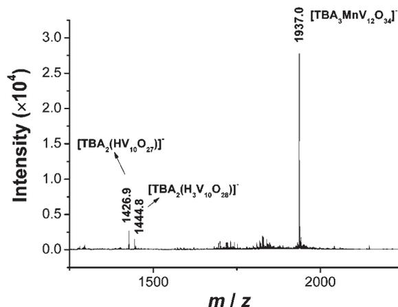
**Fig. 3** The negative ion mode mass spectrum of the product isolated from the reaction of  $\text{K}_7[\text{Mn}^{\text{IV}}\text{V}_{13}\text{O}_{38}] \cdot 18\text{H}_2\text{O}$  and TBABr in acetonitrile, showing the species related to  $[\text{MnV}_{12}\text{O}_{34}]^{4-}$  and  $[\text{H}_3\text{V}_{10}\text{O}_{28}]^{3-}$ .
