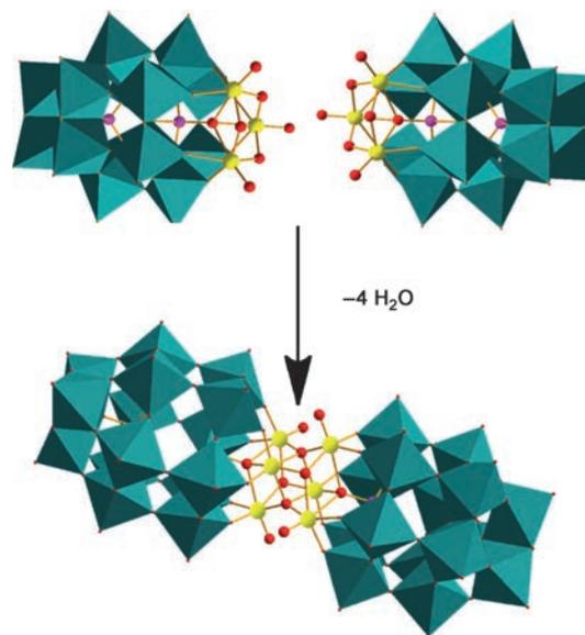
**Figure 1.** (TBA)<sub>10</sub>[P<sub>4</sub>V<sub>6</sub>W<sub>30</sub>O<sub>120</sub>] (**1**; bottom) with double cubane core. Green octahedra: WO<sub>6</sub>, pink spheres: PO<sub>4</sub><sup>3-</sup>, yellow spheres: V, red spheres: O. TBA counterions are omitted for clarity.
