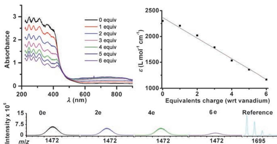
**Figure 4.** Correlation between the mass spectrum and UV/vis spectrum of **1** during electrochemical reduction. The molar extinction coefficients are calculated at 423 nm and a reference peak is used in the mass spectrum to compare the product peaks. The reference peak is assigned as  $[(TBA)_4(PF_6)_5]^-$ , which is subjected to the same experimental conditions as **1**.
