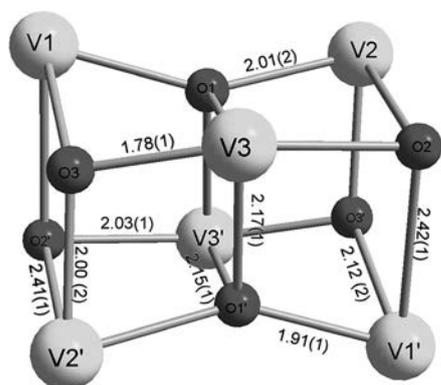
**Figure 2.** The double cubane vanadium core unit found in **1**. The double cubane core of the sandwich structure is shown with O-V-O bond lengths included. The majority of the bond angles are between 70.1° and 79.5°, with the exception of the vanadium atoms linking the cubanes, O3-V3-O2 and O2'-V3'-O3', which are 153.3(5)° and the bond lengths are between 1.92 and 2.40 Å.
