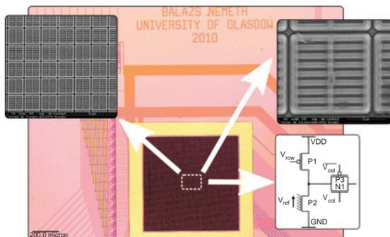
Fig. 1 Structure of pixels and micrographs of fabricated sensors and system
