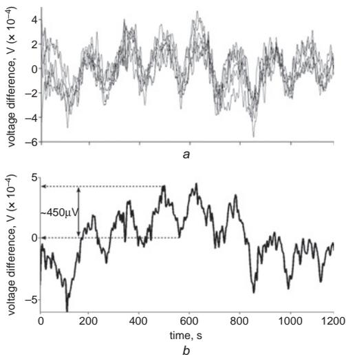
**Fig. 3** Response of five pixels shows excellent correlation (Fig. 3a) (pixels selected from four corners and one from middle of array); amplitude of pixel output voltage signals (Fig. 3b) (response of pixel located in middle of array displayed)
