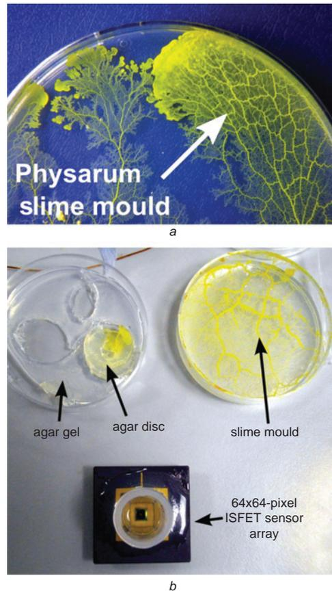
Fig. 2 *Physarum* slime mould growing on 1.5% agar gel (Fig. 2a) (slime mould shape consists of flat area in growing fronts and tubular structures in interior side of cell); slime mould was placed into plastic chamber on top of chip carrier (Fig. 2b) (agar gel deposited over cell to maintain moist environment)
