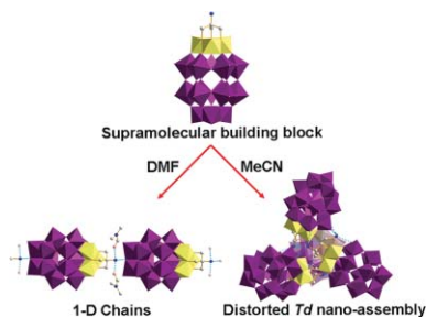
Fig. 14 Solvent dependant formation of different architectures from tris-grafted \{\text{P}_2\text{V}_3\text{W}_{15}\} clusters.
