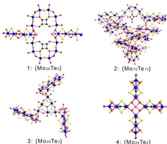
**Figure 2.** Structural representations of the four newly discovered Te-containing POTMs:  $\{\text{Mo}_{28}\text{Te}_2\}$ , 1;  $\{\text{Mo}_{72}\text{Te}_{12}\}$ , 2;  $\{\text{Mo}_{30}\text{Te}_3\}$ , 3 and  $\{\text{Mo}_{24}\text{Te}_2\}$ , 4; colour scheme: Mo-blue, S-yellow, O-red, C-black, Te-pink.
