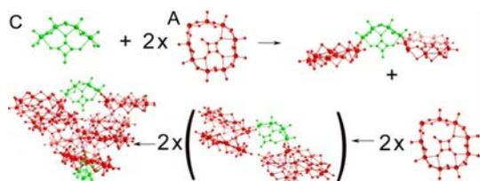
**Figure 4.** Schematic representation of the sequential build-up of **2** from the BBs, starting with two **A** connecting with a **C** unit to form the first layer, followed by two additional **A** units to form a second layer, where two of these formations assemble orthogonally to form a four-layered structure. BB **C** is denoted in green.
