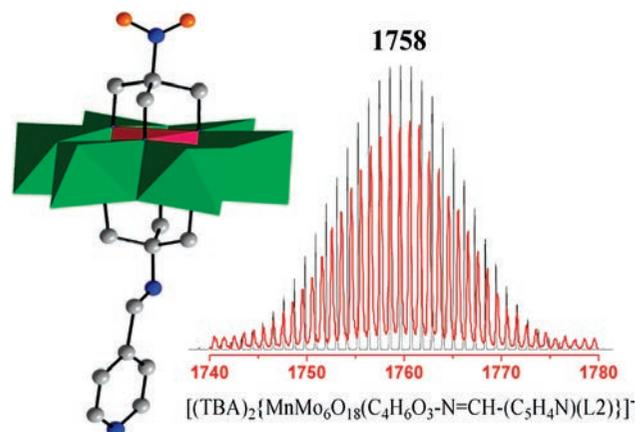
**Figure 2.** Left: X-ray crystal structure of compound **2** shown as a polyhedral representation showing that a pyridyl ring has been covalently tethered to the Mn-Anderson cluster (Mn, pink; Mo, green; N, blue; C, gray; O, orange). Right: ESI-MS spectrum of the molecular ion peak of compound **2** (actual spectrum in red; calculated spectrum in black).
