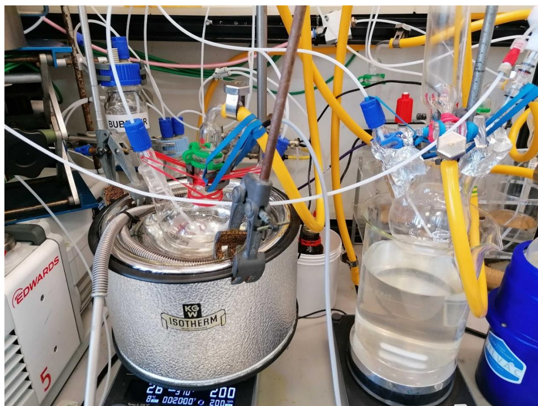
Figure S21: Coupling flask with chiller setup to cool a dewar of acetone.
