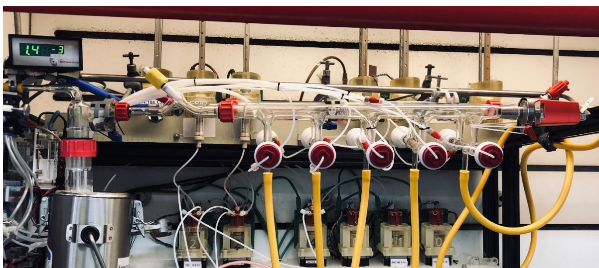
Figure S33: Assembled AutoSchlenk Line with Liquid N 2 Trap and attached Vacuum pressure gauge.
