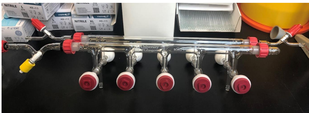
Figure S32: AutoSchlenk glass manifold with 5 ports on each line of vacuum (front) and inert gas (back).
