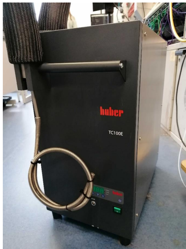
Figure S6: Huber TC100E immersion cooling chiller.
