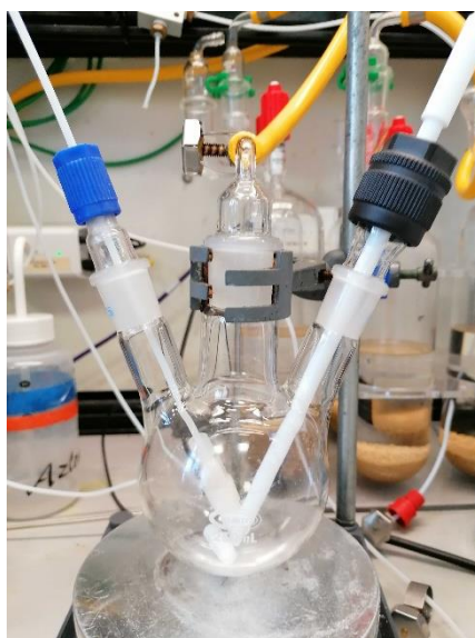
Figure S48: Example setup of 3-necked RBF with temperature probe.
