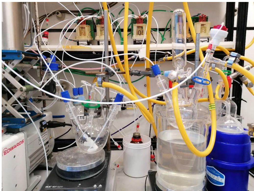
Figure S20: Full setup showing Coupling Flask (LHS) and the Evaporating Flask (RHS), above a paraffin oil bath, which is shown in more detail below.
