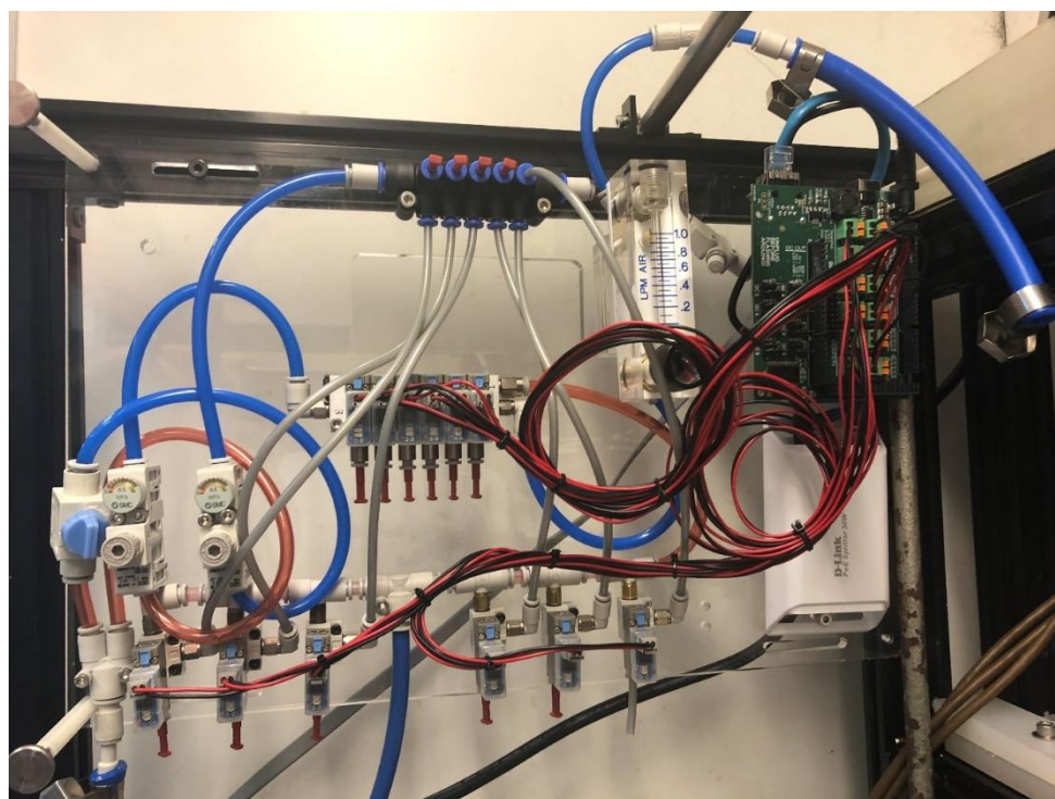
Figure S39: Photograph of the solenoid manifold without outlet tubing as built.
