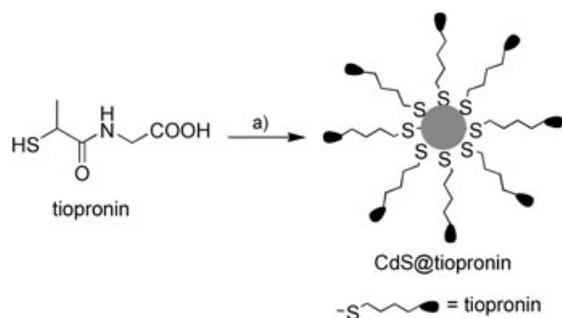
**Scheme 1.** Preparation of CdS@tiopronin: a) Cd(NO<sub>3</sub>)<sub>2</sub>·4H<sub>2</sub>O, Na<sub>2</sub>S, pH 10, H<sub>2</sub>O.
