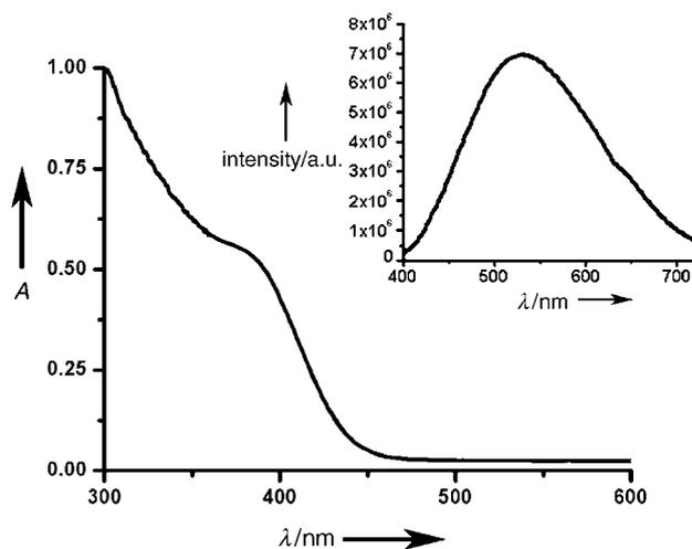
**Figure 1.** UV/Vis and fluorescence (inset;  $\lambda_{\text{exc}} = 380$  nm) spectra of CdS@tiopronin in water.
