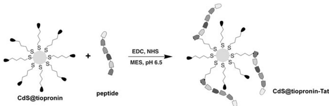
**Scheme 2.** Synthesis of CdS@tiopronin-Tat. NHS = *N*-hydroxysuccinimide (5 mM), EDC (2 mM), MES = 2-morpholinoethanesulfonic acid (pH 6.5).
