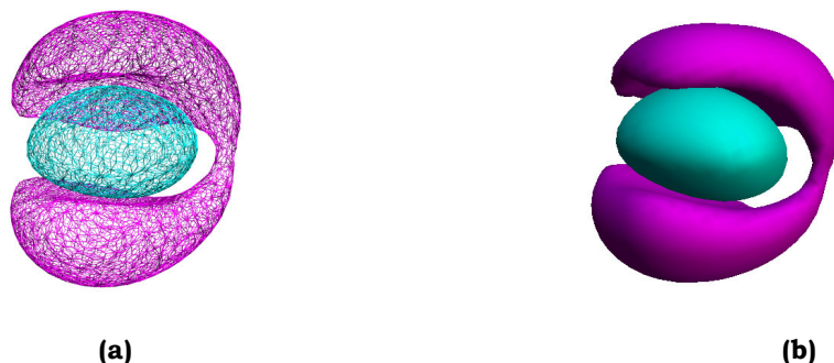
Fig 11-1 Illustrative iso-surface plots of the density modification from the 3rd and 4th order anharmonic components to a pdf, showing the positive (cyan) and negative (magenta) regions. The graphical programs used were (a) MCE [6] and (b) XDGRAPH.
